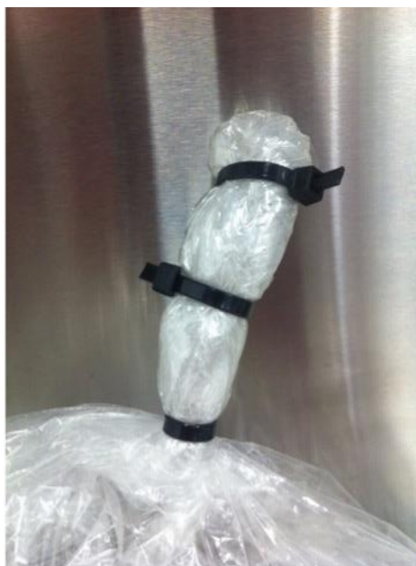
Well-sealed plastic bag: twisted shut, gooseneck tie, cable ties, and tape.
