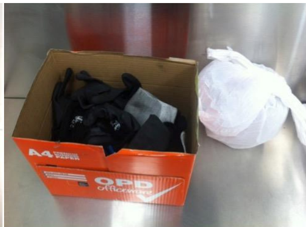
Inappropriate fire debris packaging: cardboard boxes and regular plastic shopping bags.
