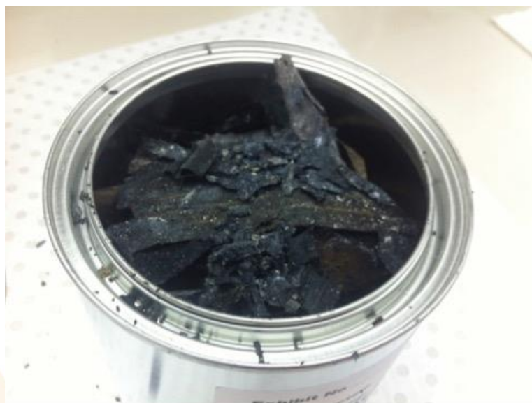
Do not overfill sample containers. This tin is too full.
