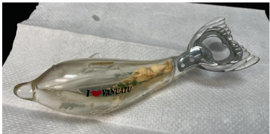
lamp oils. This result helped explain the petroleum-like odour that the client encountered when they touched the fluid which was leaking from the bottle opener.
